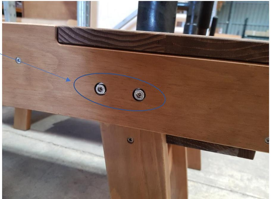
STEP 2: Remove the pump lever but taking out the little screws – can be a bit fiddly. :)
