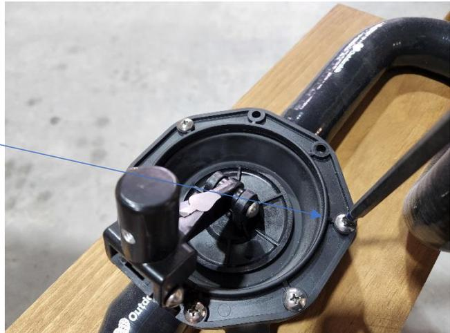
STEP 6: Remove the flange housing from the pump.
