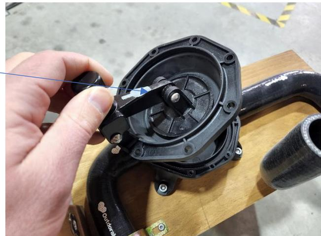
STEP 5: Remove the centre screw holding the flange on.
